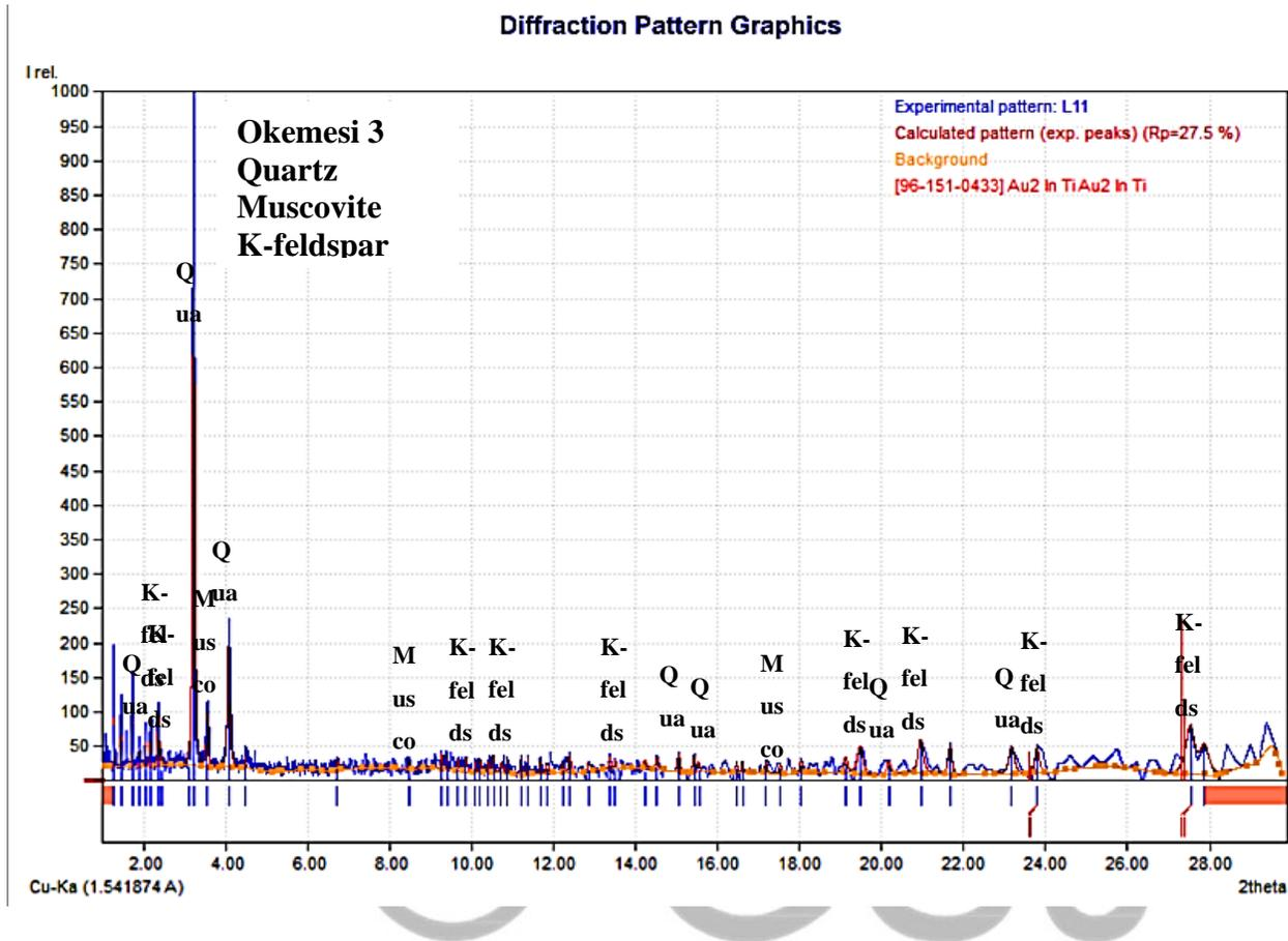
Figure 57: X-ray Diffractogram of Okemesi 3 Quartzite. (Location N7°49.854' E4°54.985')
