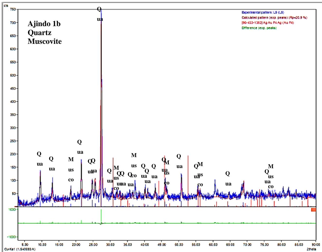
Figure 55: X-ray Diffractogram of Ajindo (1b) Schistose quartzite (Location N7°52.381' E4°57.535')
