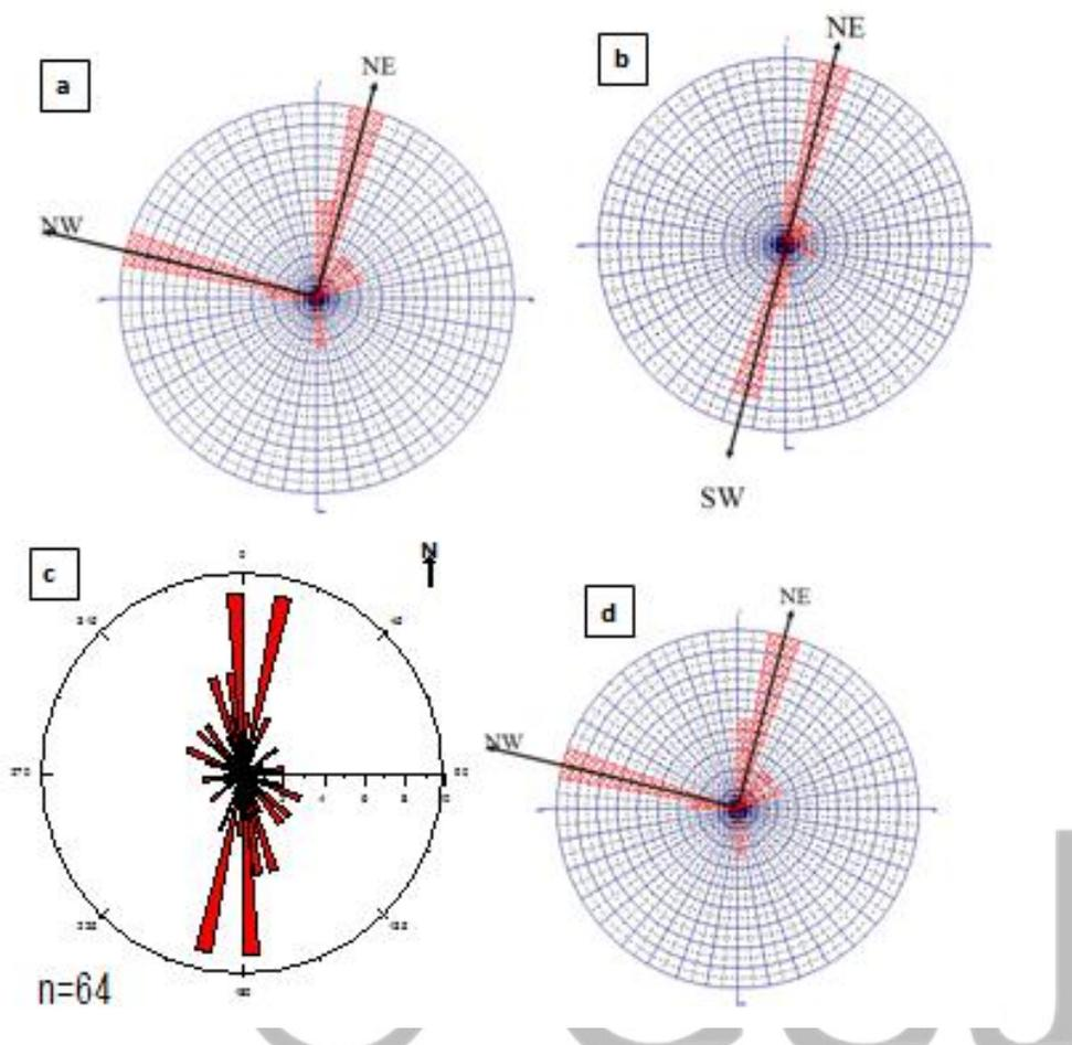
Figure: (a) Rosette diagram of Joints orientation in the study area; (b) Rosette diagram of veins orientation in the Study Area; (c) Rose plot showing fractures trend in the study area; (d) Rosette Diagram of Joint trend in the Study Area.
