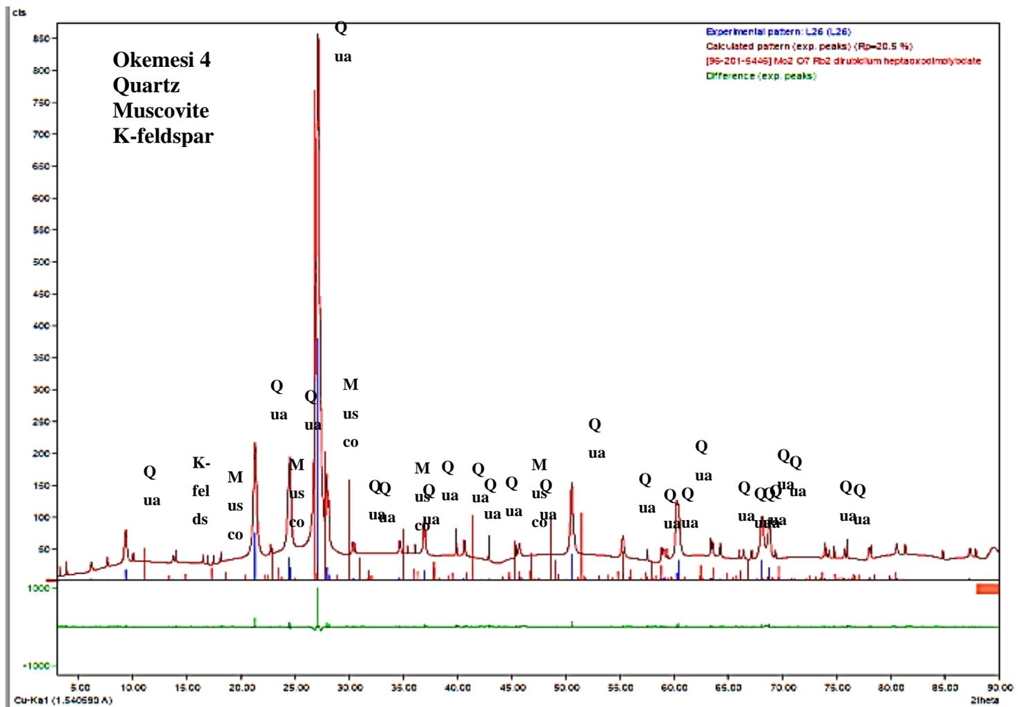
Figure 58: X-ray Diffractogram of Okemesi 4 Schistose quartzite. (Location N7°50.340' E4°54.832')
