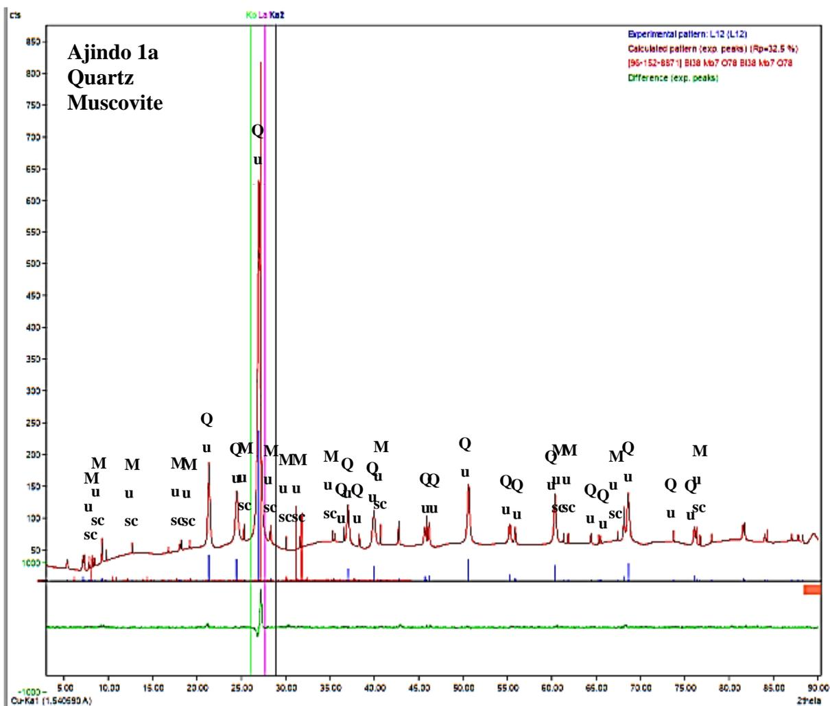
Figure 54: X-ray Diffractogram of Ajindo (1a) Schistose quartzite (Location N7°52.354' E 4°57.496')
